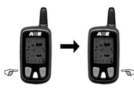
Pressing button 1 immediately before button 2 is pressed will disarm the alarm system without beeping the siren unit. All other features including the indicator flashes will remain the same. Note: If the alarm is giving the driver a warning such as four flash warning that the alarm has been triggered, the alarm system will beep the siren even if it is overridden by the remote or the software switch. Fault warnings take priority over silent disarming.
