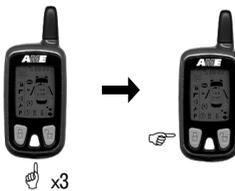
The transceiver includes an internal Vibrator to indicate a zone trigger or pre-warn input. The Vibrator can be turned ON and OFF by pressing button 3 three times followed by Button 1. If you turn off the vibrator, all vibrating confirmation/warning will be cancelled. Turning on the vibrator the transceiver will confirm with a vibrating signal and all vibration signals will work as normal.
