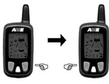
Pressing button 2 immediately before button 1 is pressed (within 3 seconds) will arm the alarm system without beeping the siren unit. All other features including the indicator flashes will remain the same. Note: If the alarm is giving the driver a warning such as three beeps for door/hood/trunk open the alarm system will beep the siren even if it is overridden by the remote or the software switch. Fault warnings take priority over silent arming.
