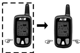
The alarm system includes a Calm Alarm Mode that will allow the alarm system to be armed in a silent mode. If the alarm system is triggered when the system is in this mode then the siren will not sound. If the alarm system is triggered, the indicators will flash as normal to show that the alarm system has been triggered. You will be informed as normal via the 2-way LCD transceiver (The device that triggered the alarm system will be identified on the LCD display).
