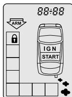
*If the engine has been started up successfully LCD Handset will display the engine running. In case of fault start the Handset will provide a warning beep.*
