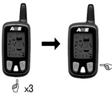
The transceiver includes an internal Buzzer and a different tone is used to indicate each different zone trigger or pre-warn input. The buzzer can be turned ON and OFF by pressing button 3 three times followed by Button 2. If you turn off the buzzer, all audible confirmation/warning will be cancelled. Turning on the buzzer the transceiver will confirm with the buzzer activation melody and all audible signals will work as normally.
